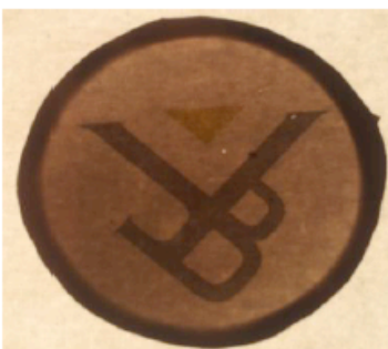
Figure 2. Semi-Transparent 30 \mu\text{m} film 0.4 wt% Loading MWCNT; 6 S/m
